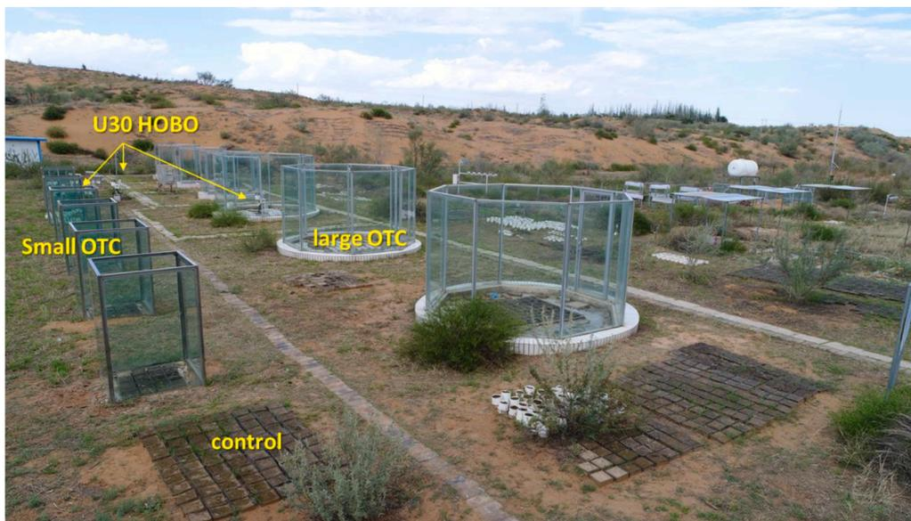
**Fig. 1.** Open-Top Chambers (OTCs) of different size were employed to simulate warming (photo in 2007). Large OTCs increase temperature by 0.5°C and reduce annual precipitation by 5%, small OTCs increase temperature by 1.5% and reduce annual precipitation by 8% in comparison with control.
